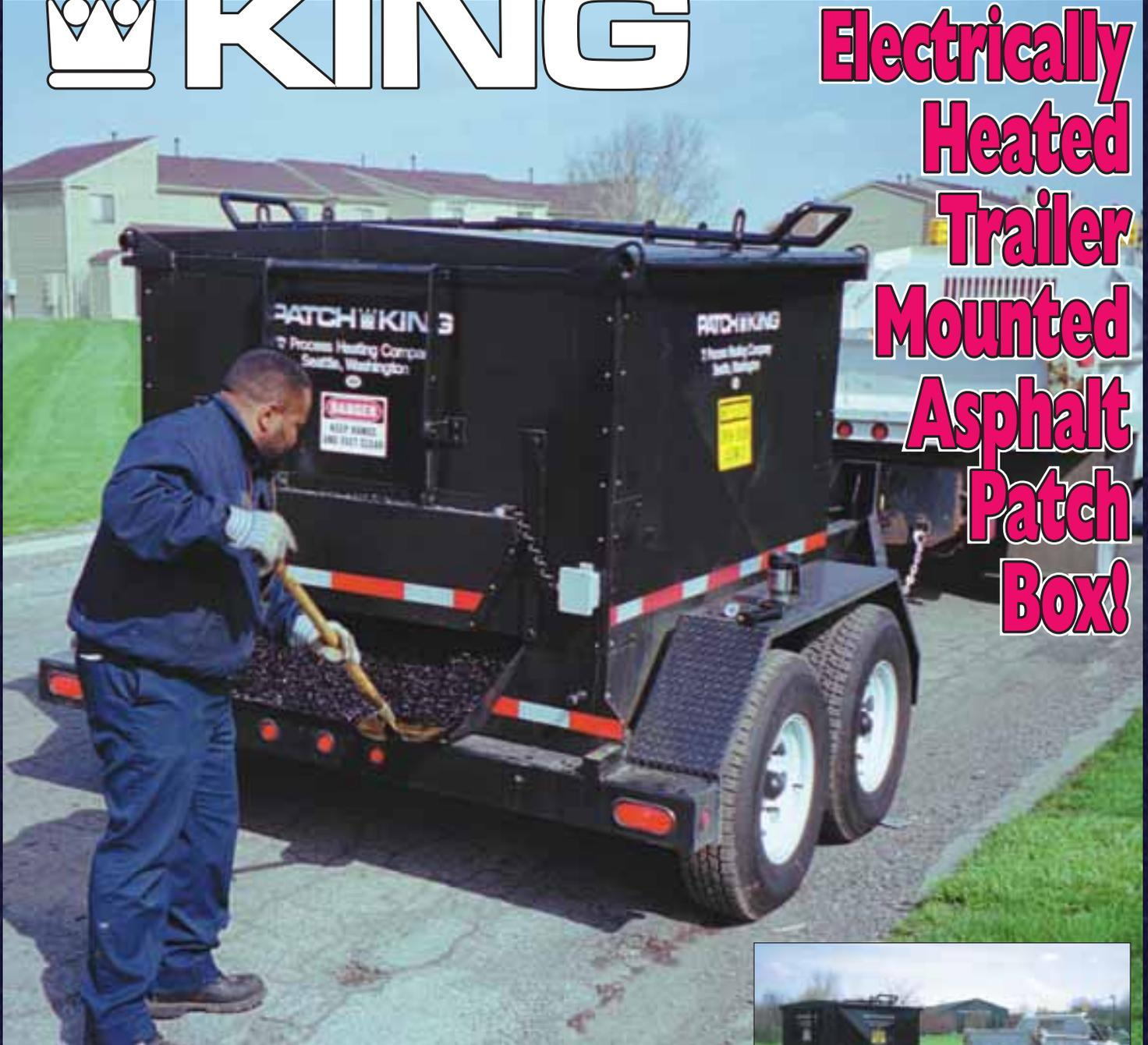
**The First Trailer Mounted Patch Box with Electric Heat for Hot or Cold Mix!**
