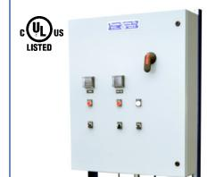
STATE OF THE ART CONTROLS - A seven day programmable clock starts the heating process automtically. The main disconnect circuit breaker de-energizes power when the panel door is open. Overcurrent Protection is the result of individually fused heat circuits. The motor is overload protected as well. Controls are U.L. listed.
